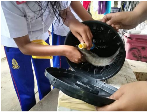
Picture 4. Testing a prototype of an automatic scale remover machine.
